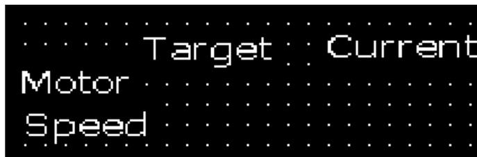
Select “Register” under “Object” menu or click
