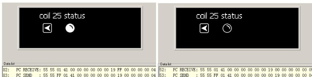
When writing coil M25 status the data format of query message from TD-43B and response message from controller is shown as following:
