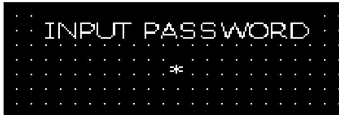
Input the password (0-999999), which is shown as"\*". Press ENT. If password is correct, it will show the window as follows:
