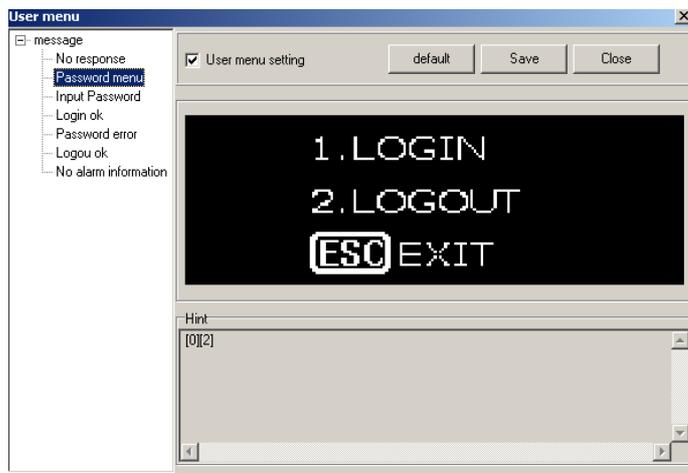
The password set interface includes “LOGIN”, “LOGOUT”, “ESC EXIT” (default information). If the text of the information in the screen need to be changed and the position need not to be changed, cross “user menu setting” check box and double click the text needed to be changed, the following prompting frame will be displayed as the following:
