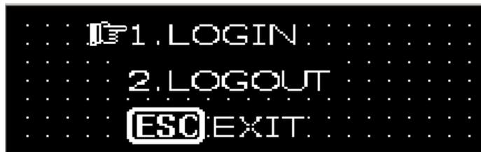
**Example:** Substitute the text “ENTER” for “LOGIN”, “QUIT” for “LOGOUT” and “RETURN” for “EXIT”. Click “OK”, the following diagram will be displayed.
