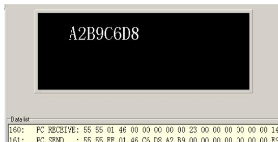
When reading Register 35 36 the data format of query message from TD-43B and response message from controller is shown as following:
