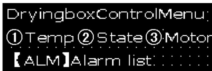
Window No.1 is a main menu window. Pressing ① switch to the window of temperature setting(No.2) that is shown as follows:
